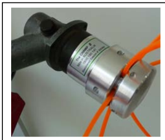
Fig 4 : 25 mm Riser on Bearing Cover
