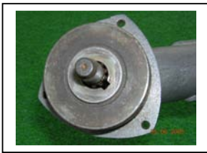
Fig 4 : 25 mm Riser on Bearing Cover
